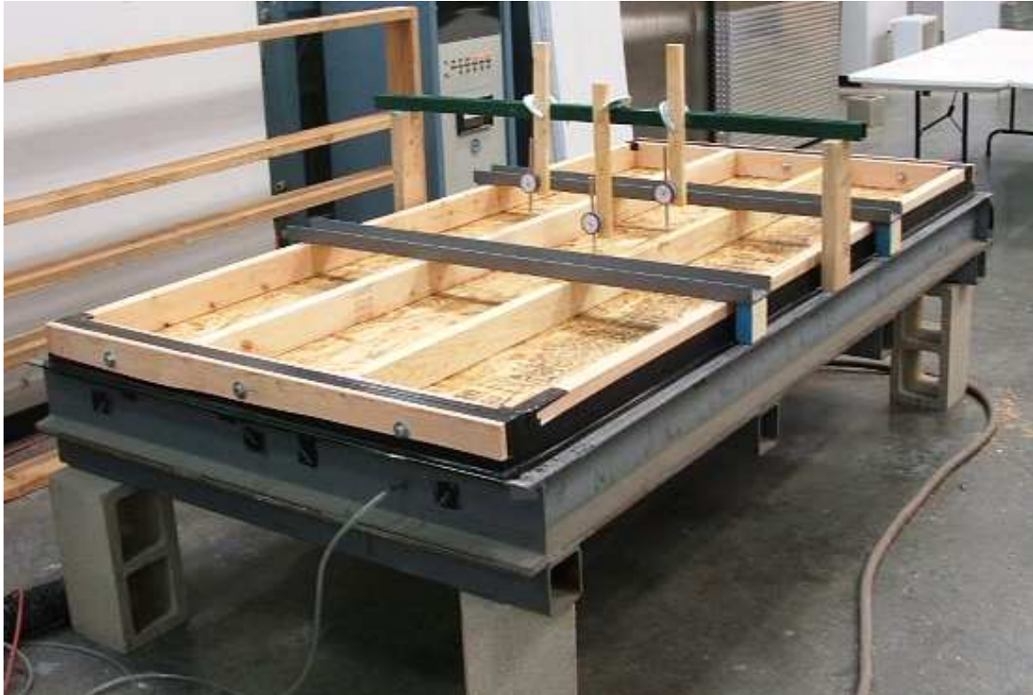
Photograph No.2 Negative Load Test Set-Up
